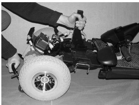
8. Press down on the rear bumper to pivot the scooter's rear section upwards until the rear section is standing vertically on its rear bumper.
