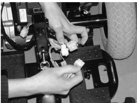
7. Unplug the front-to-rear harnesses. On the Vitesse 8 only, remove the 'R' clip and pin attaching the rear cable brake.
