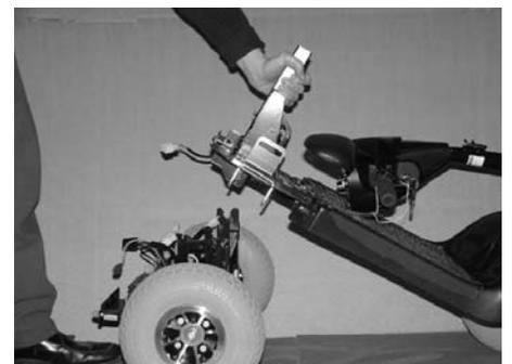
9. Lift the front section until the lower pegs are no longer in the curved locking brackets. Carefully lift the front section away from the rear section.
