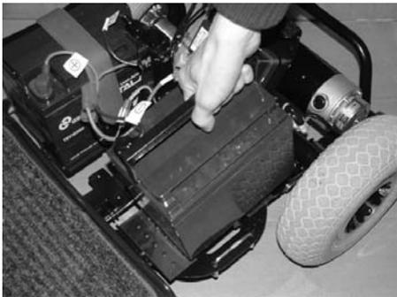
4. Undo the Velcro straps and remove batteries.
