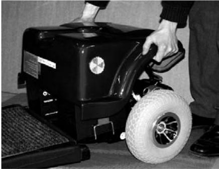
1. Switch off the scooter, unscrew the seat hand wheel and remove seat. Be careful not to let the seat post drop when removing.
