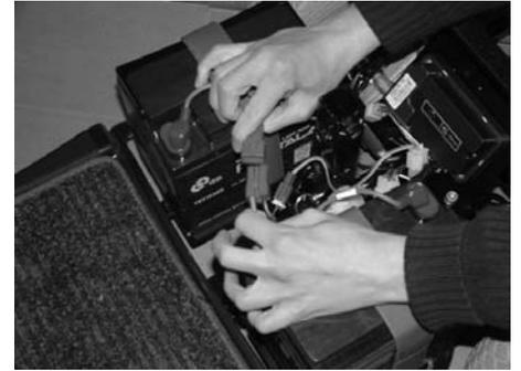
3. Disconnect the batteries by disconnecting the two red connectors and two black connectors.
