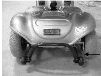
Push the freewheel lever down completely and the scooter can be moved manually. (See photo left)
