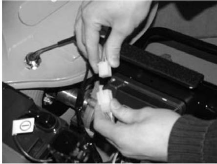
2. Lift up the rear shroud to remove. Disconnect the rear lamp connector to allow this.
