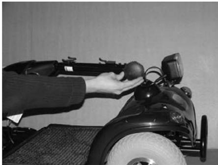
5. Loosen the tiller adjustment knob and fold down the tiller and retighten knob.
