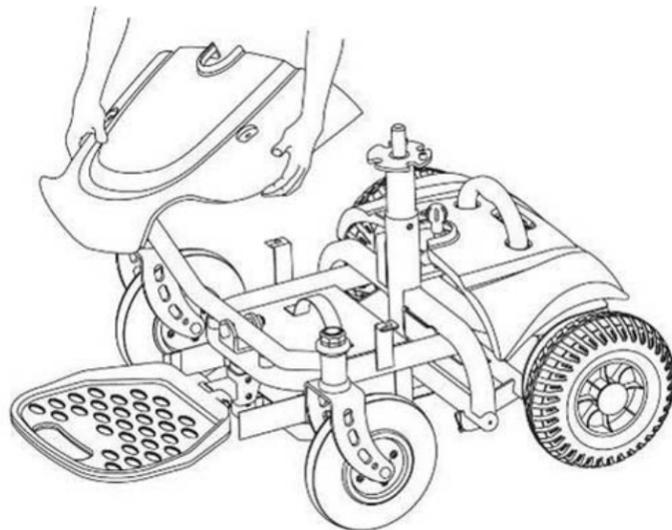
7. Lift the seat and pull the swivel lever up at the same time. Lower the bottom of the seat onto the seat post. Release the lever, swivel the seat and push down on the seat until it locks in place.
