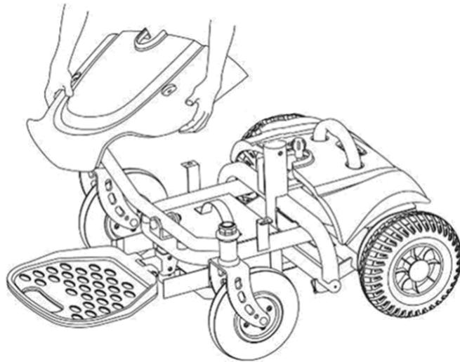
3. Install the seat post. Ensure that the seat post is aligned so that the two flanges with holes are facing the rear of the product. Having these flanges rotated into any other position will result in instability in the seat.
