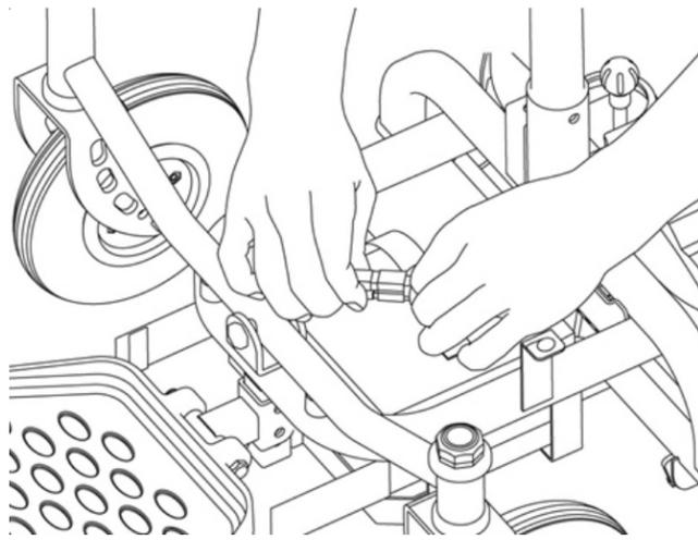
6. Replace the cover shroud. Replace and tighten the two knobs removed in Step 1.
