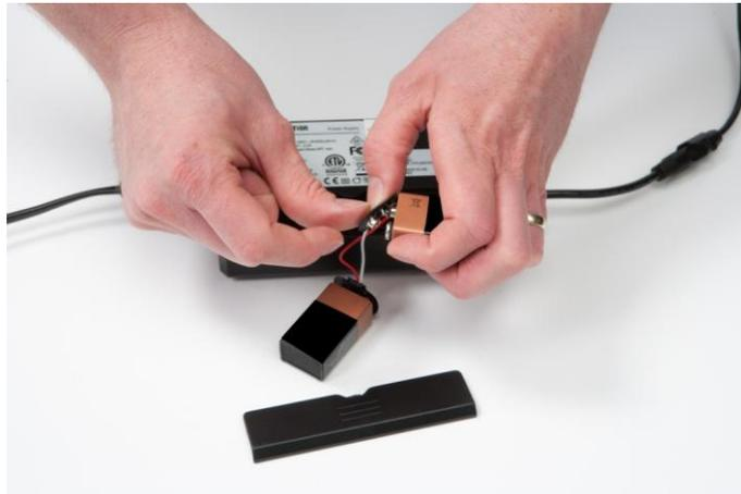
2. Pull out the two battery connectors from the compartment in the power supply and push a 9V battery on to each of the connectors.
