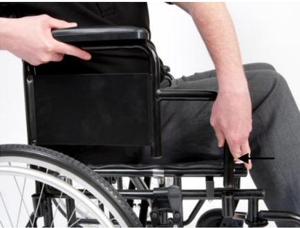
To remove the arm rest, please the chrome button at the front of the armrest (arrowed) and pull up on the armrest.
