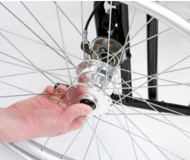
The Sentra fitted with cable brakes also feature quick release wheels. To remove the wheels, press the button in the centre of the wheel whilst pulling the wheel away from the wheelchair. To add the wheel, press the button whilst reinserting the quick release pin in to the wheelchair frame.
