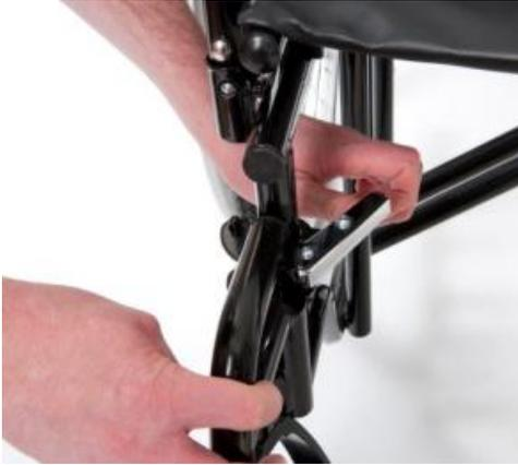
To remove the leg rest, press the chrome lever on the leg rest whilst swinging the leg rest out (as shown left). This will now allow the leg rest to be lifted up and removed. To attach the leg rest, place the leg rest on the two receiver posts on the wheelchair frame. Then swing the leg rest inwards until it locks in position.
