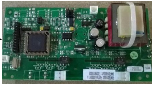
16 PCB Main inc EPROM Chip Programmable for Pump1000 1009980025
