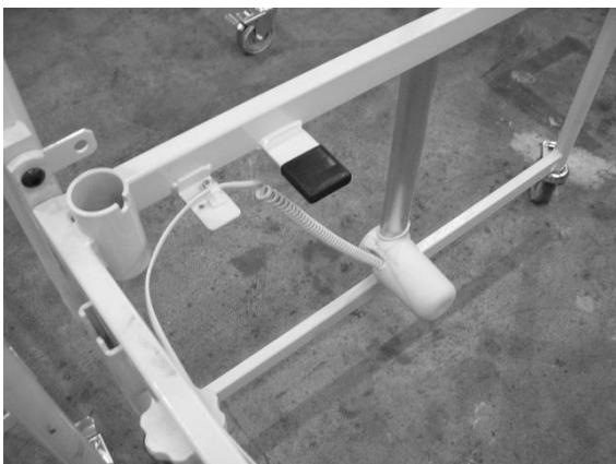
Cable to the motor at the head end of the bed.
