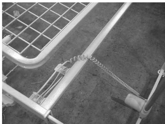
**INCORRECT** method of fitting the cable, foot end.
