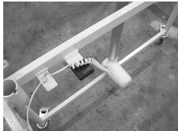
**INCORRECT** method of fitting the cable, head end.
