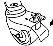
Once the bed is sited in the desired position, always ensure that the castors are locked in the braked position (see illustration)
