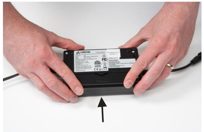
4. Slide the battery compartment lid back on to the power supply.
