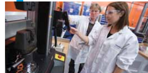
↑ President's scholar Tereze setting up a 50kN universal test machine for a tensile test of a composite specimen
