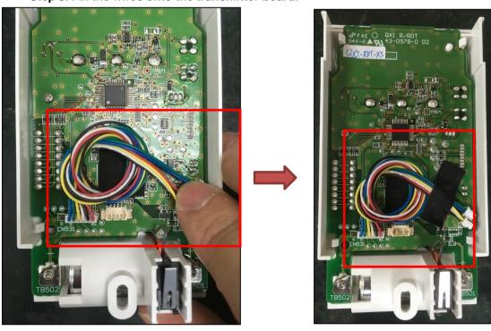
Step 6. Fix the other pair of wires onto the area below the battery case. (Refer to the pictures below)
