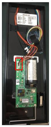
Note: The front of the device should look like this when the transmitter is installed. Full rotation of the front will not be interfered by the wire connection.
