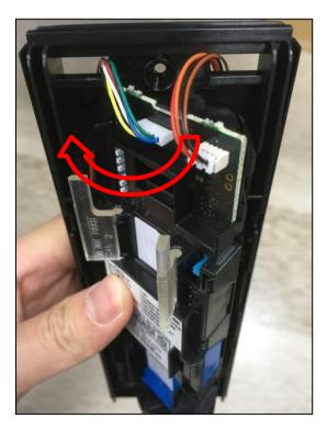
Step 5. Pull the cables downward and paste the cables onto the device.
