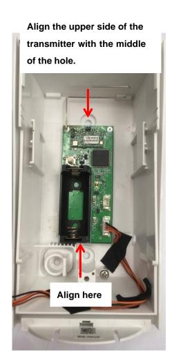
Step 3. Connect the wires and fix the wires as the pictures shown below.
