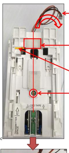
Turn the BXS-RAM around. Use the wires to make a loose knot and thread the wires' end into the circles.
