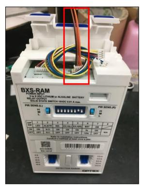
Step 4. Turn the BXS-RAM around. Use the wires to make a loose knot and thread the wires' end into the circles. Apply a foam tape to fill in the gap as the picture marked below. Align the transmitter in the middle of the back cover as the picture shown below.
