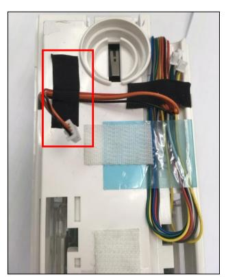
Step 7. To install the transmitter, the lower side of the transmitter should be align the installation line and use the middle of the hole or the middle of the screw to align the transmitter in the middle. Please refer to the pictures below.
