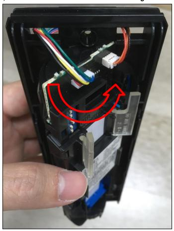
Step 3. Turn to the back of the board. Use the wires to make a loose knot, and thread the wires' end into the circles.
