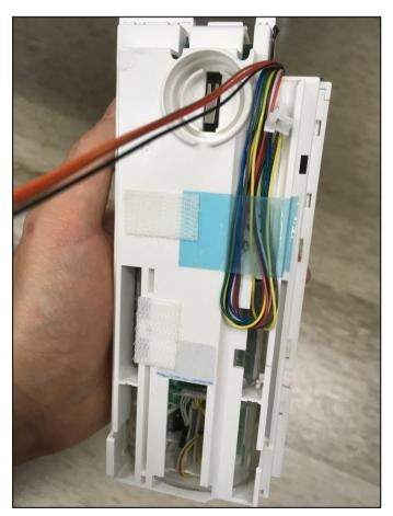
Step 5. Then, take the wires connected to the small board, and fix them onto the device.
