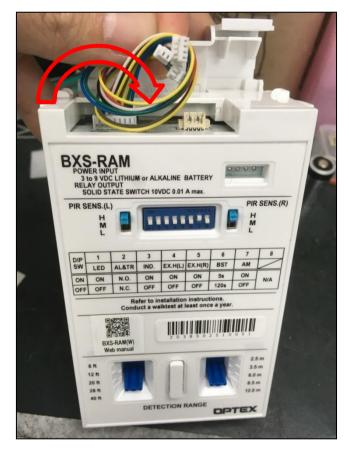
Step 3. Thread the other pair of wires through the knot, and fix the wires onto BXS-RAM.
