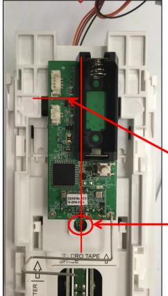
Align the lower side of the wire connector here.
