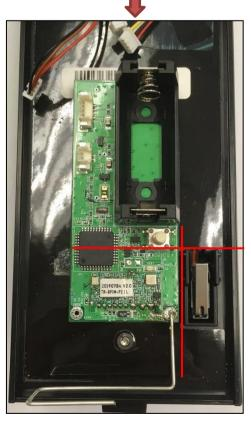
Step 8. After installing the transmitter, connect the cables. It should look like the picture below when the installation is completed
