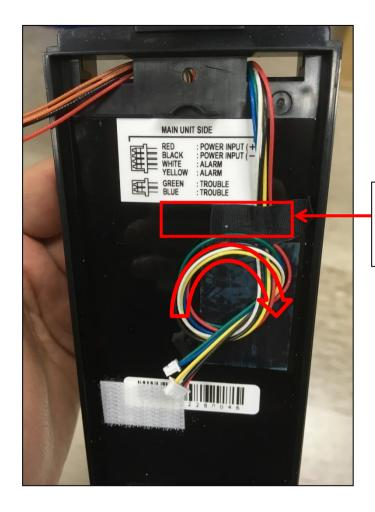
Be sure to paste the wires under the sticker to avoid blocking the label.
