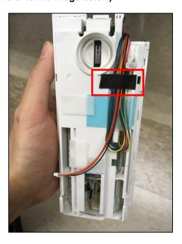
Step 6. Fix the rest of the wires onto the device.
