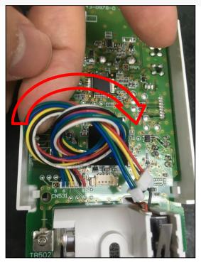
Step 5. Fix the wires onto the transmitter board.
