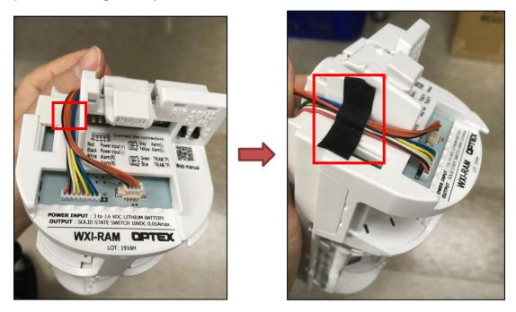
Step 4. Bend the wires that are not connected to the small board, and fix it onto the device.
