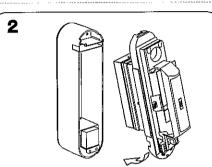
After cabling between transmitter and the unit can be fixed with 2 screws. Hook the unit onto the BACK BOX fasten turn 2 lock screws on the unit below.
