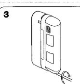
Put the cover on and conduct walk test. After completed turn the lock screw on the cover.
