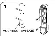
Use the MOUNTING TEMPLATE. Then hold the template against the mounting surface, when BX-80NR is to be mounted. Mark the position of the mounting hole then discard template. Then fasten the unit on the marked position.
