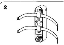
Use the metal strap to fix the unit. Tightly strap the unit on a gutter. (Max strap size: Width 20mm / Thickness
