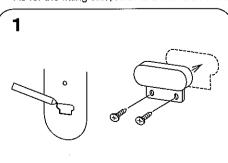
Use the enclosed MOUNTING TEMPLATE to determine where it is to be installed.
