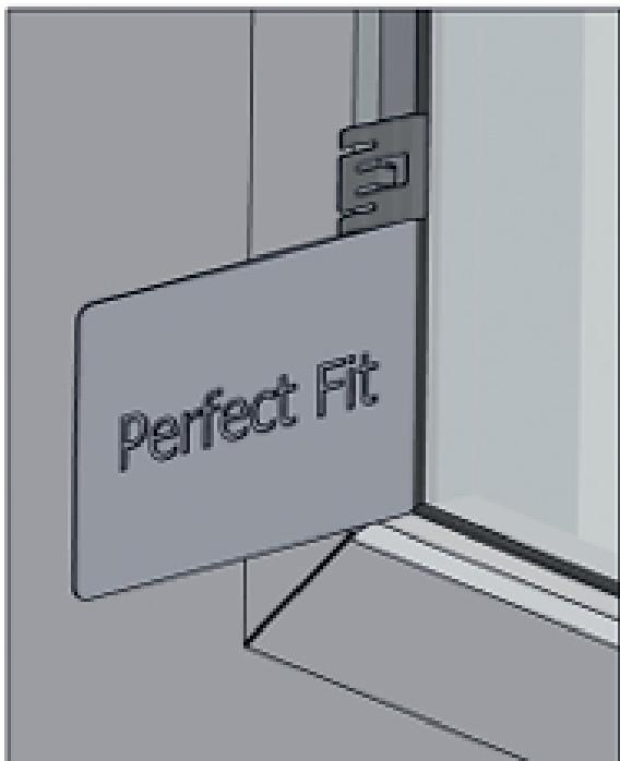
To ensure all the brackets are in the correct position for fitting use the 85mm side of the fitting card for the bottom brackets. Please use 122mm side of the card for the top brackets.
