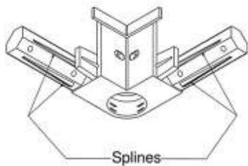
Use the push fit corner pieces to join the side rails to the top and bottom frames of the blind. Simply push them into the slots in the frame pieces to lock them into place.
