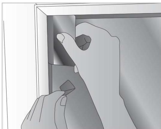
You need to push the brackets between your window pane and the rubber window seal.
