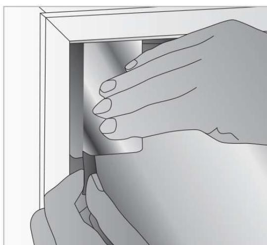
Fit any intermediate brackets accordingly. Two extra brackets will be supplied for blinds over 120cm drop, these should be positioned approx mid way down the drop of the blind one on each side. These need to be lined up with the bracket hole positions on the Perfect Fit frame.
