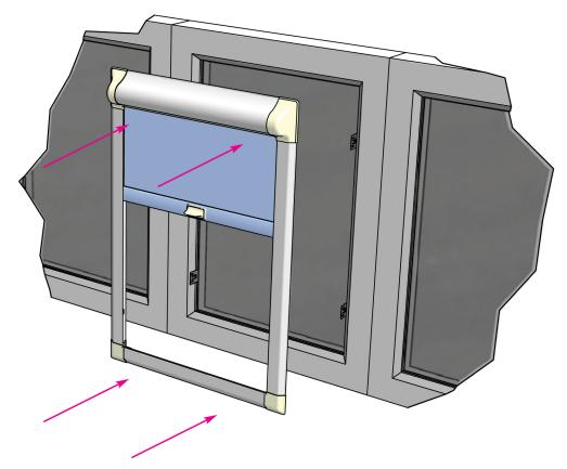
Firmly press the frame down onto each bracket. Fit one side at a time for an easier installation.
