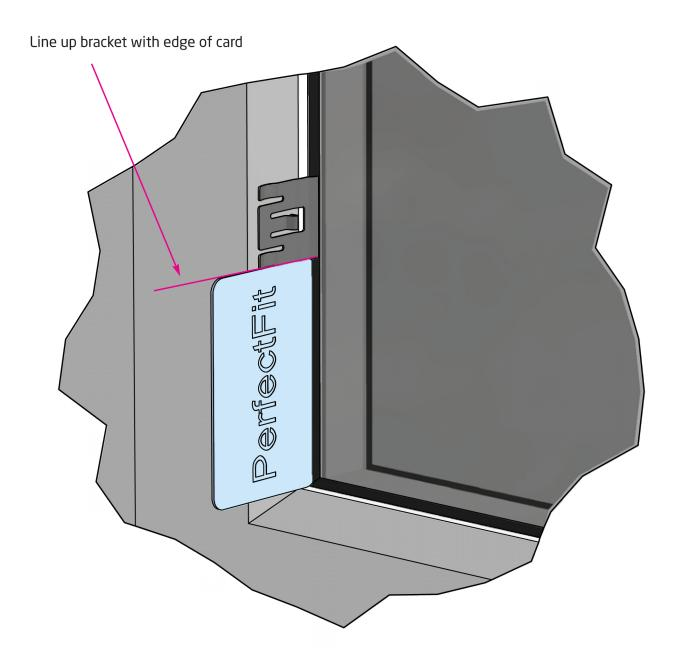
Line up the bracket with the base or top of the credit card (depending on which corner of the window you are working) and fit the bracket by pushing it between the glass and the rubber seal of the window.
