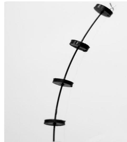
Figure 5: Articulation joint structure using the common beam and disk arrangement to achieve tool positioning.
