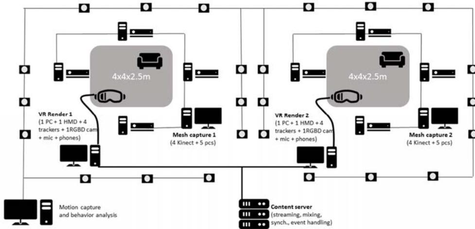
Figure 5. Composition of each of three lab nodes that form part of the distributed VR-Together User Lab.
