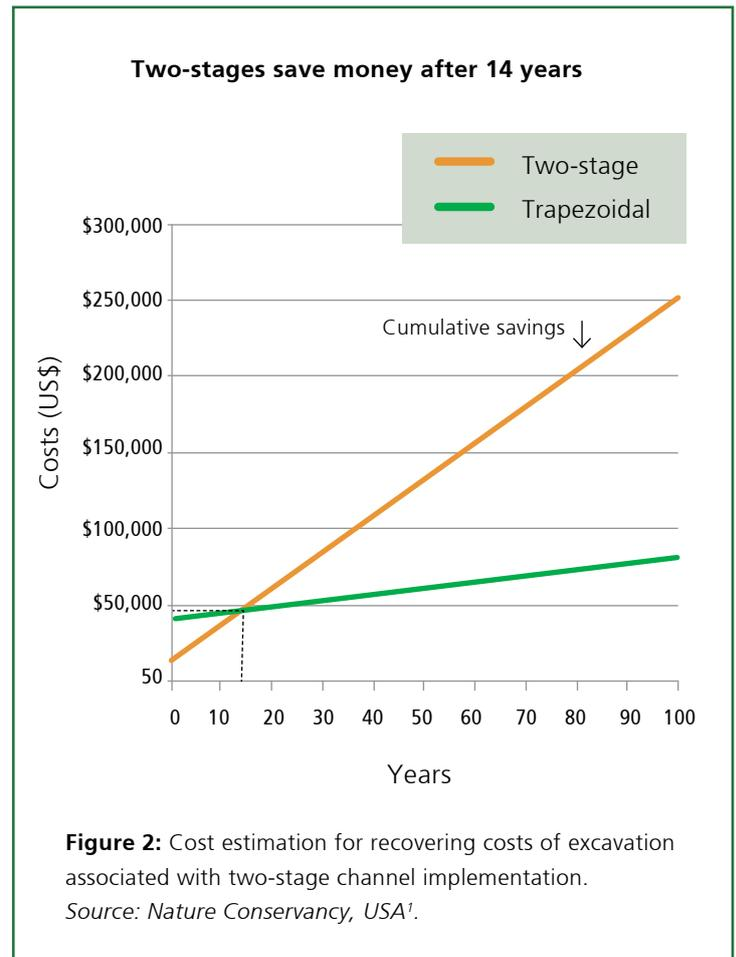
**Figure 2:** Cost estimation for recovering costs of excavation associated with two-stage channel implementation. Source: Nature Conservancy, USA<sup>1</sup>.
