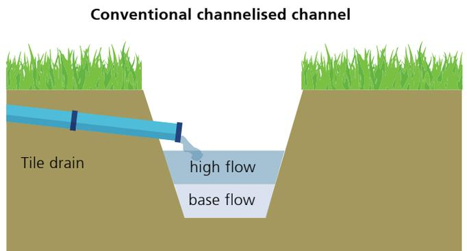
Figure 1a. Cross-section profile of a conventional channelised channel.
