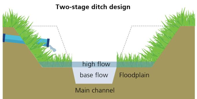
Figure 1b. Cross-section profile of a two-stage channel design<sup>5</sup>.
