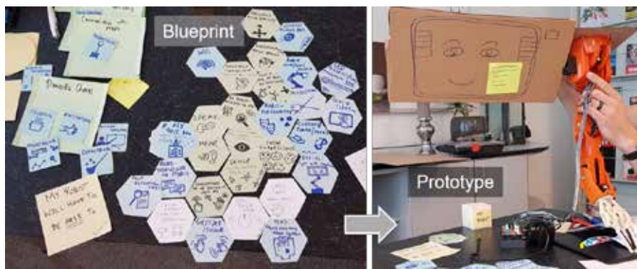
Figure 6. Tom designed a cooking assistant with a digital face, an interactive touchscreen and an arm for cooking-related tasks
