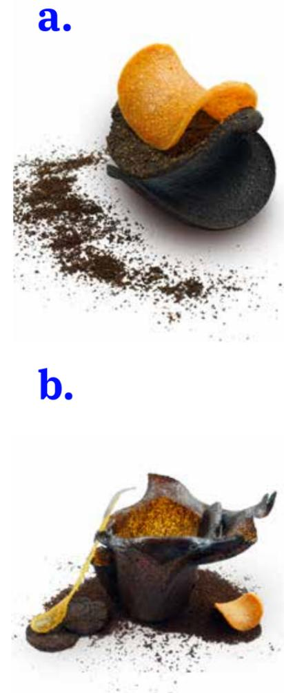
**Figure 1a, b.** Gelatine bioplastic samples. Exploring material limitations and possibilities in creating design artifacts. Photo: Jekaterina Aleksejeva.
