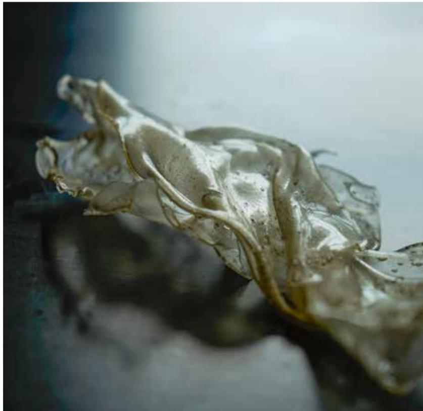
**Figure 3.** Bioplastic foil. Some of the samples produced, showed that bioplastics can create a variety of outcomes – from solid samples to foils and flexible materials. Photo: Paul Biedermann.
