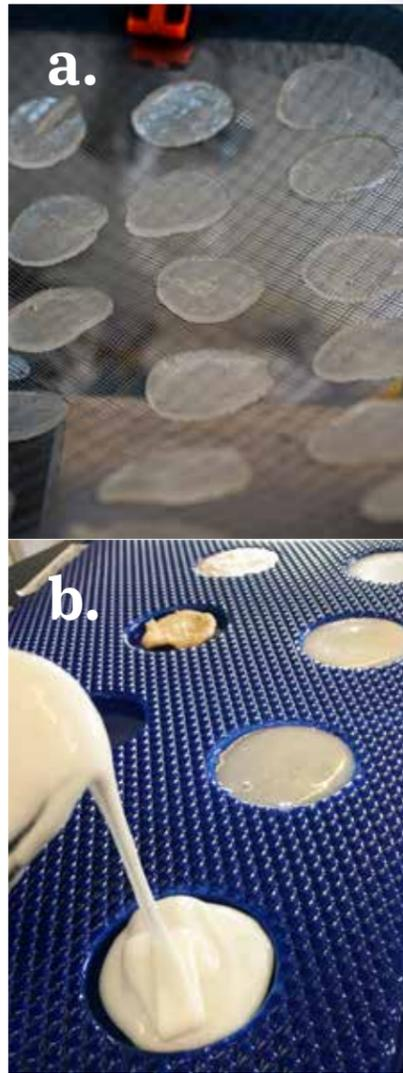
**Figure 2a.** Agar bioplastic samples during casting. The material almost fully dissolved during the casting process. Photo: Paul Biedermann. **Figure 2b.** Vacuum formed plastic sheets. Used for casting and organizing bioplastic samples. Photo: Paul Biedermann.
