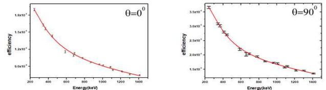
Fig.3 The efficiency curves of the detectors at  $0^\circ$  and  $90^\circ$  along with the experimental data.
