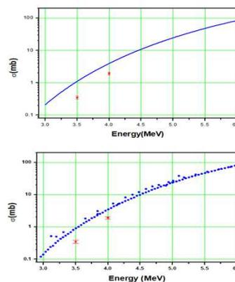
Fig. 5 Experimental cross sections compared with the bibliography data (bottom) and the results from TALYS code (top).
