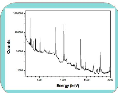
Fig. 2 Typical spectrum of a HPGe detector at beam energy 4 MeV
