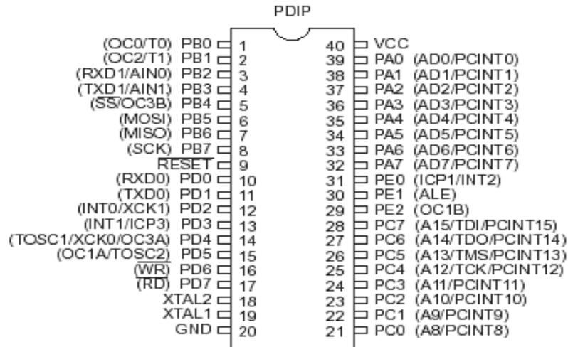
Figure.3 Pin diagram of ATmega162 Microcontroller
