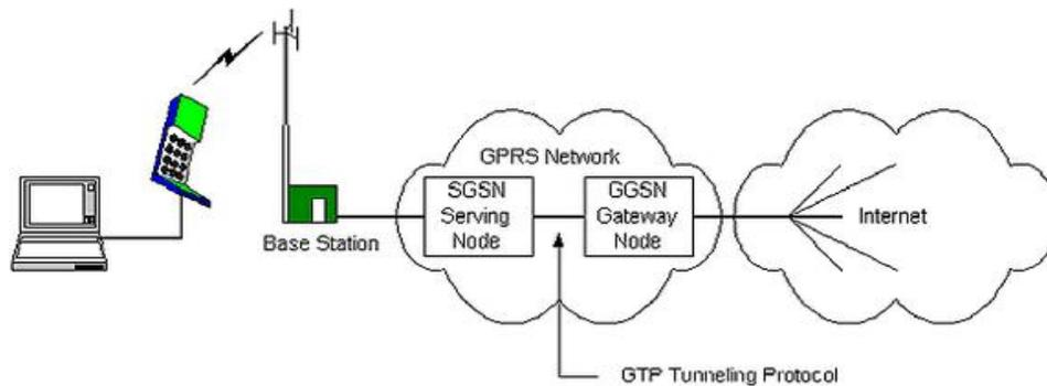
Figure.1 Schematic diagram of GPRS
