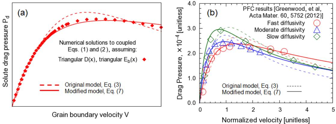
Fig. 3: (a) The drag pressure data from Figure 1(c), now being fit to the modified solute drag model. (b) The PFC simulation results from the literature [11] on the drag pressure variation with velocity for different solute diffusivities, being fit to both the original and the modified solute drag models.
