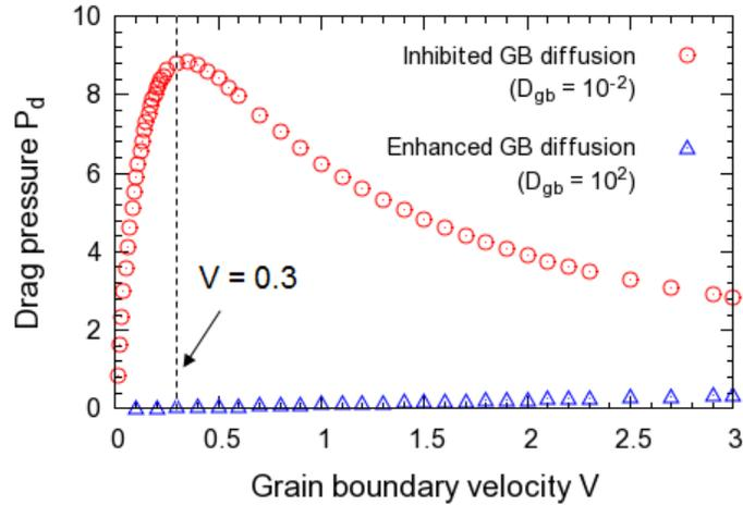
Fig. 6: The dependence of drag pressure on grain boundary velocity for two cases of solute diffusion: inhibited diffusion and enhanced diffusion at the boundary. For  $V \leq 0.3$ ,  $P_d$  increases with increasing  $V$ .
