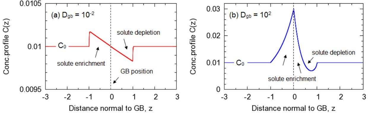
Fig. 7: The concentration profile at steady state for (a) inhibited solute diffusion at the boundary, and (b) enhanced solute diffusion at the boundary.
