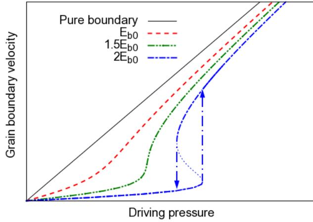
Fig. 2: The velocity-driving pressure relationship predicted by the Cahn solute drag model under different binding energies. The curve labelled ' $2E_{b0}$ ' illustrates a hysteresis denoting different paths for abrupt break-away transitions, the dotted part representing the so-called unstable regime.
