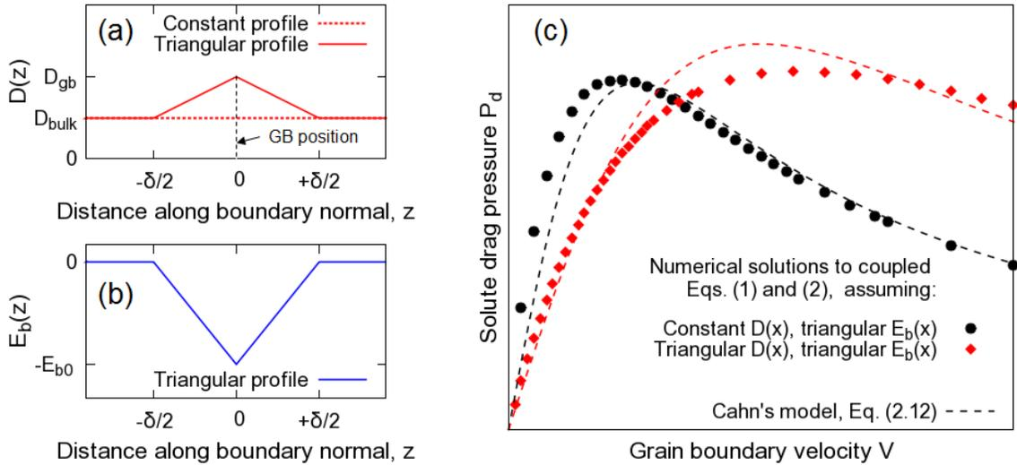
Fig. 1: Examples of (a) diffusivity profiles  $D(z)$  and (b) binding energy profile  $E_b(z)$ ,  $\delta$  and  $E_{b0}$  being the grain boundary width and the maximum binding energy, respectively, (c) solute drag pressure dependence on boundary velocity; data points are the solutions to Eqs. (1) and (2) while the dashed lines are the model from Eq. (3).
