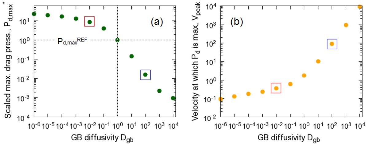
Fig. 5: Variation of (a) the scaled maximum drag pressure  $P_{d,max}^*$  and (b) the peak velocity  $V_{peak}$  with grain boundary diffusivity  $D_{gb}$ . The scaled maximum drag pressure  $P_{d,max}^*$  is the ratio between the maximum drag pressure for a given  $D_{gb}$  and the reference maximum drag pressure, i.e.  $P_{d,max}^{REF} = P_{d,max}(D_{gb} = D_{bulk}=1)$ .
