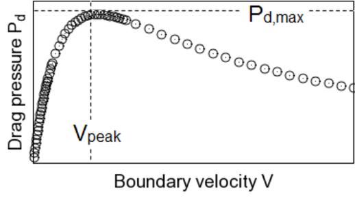
Fig. 4: A plot of drag pressure vs grain boundary velocity obtained from solving Eqs. (1) and (2) numerically. The maximum drag pressure  $P_{d,max}$  and the corresponding velocity (or peak velocity)  $V_{peak}$  are highlighted.
