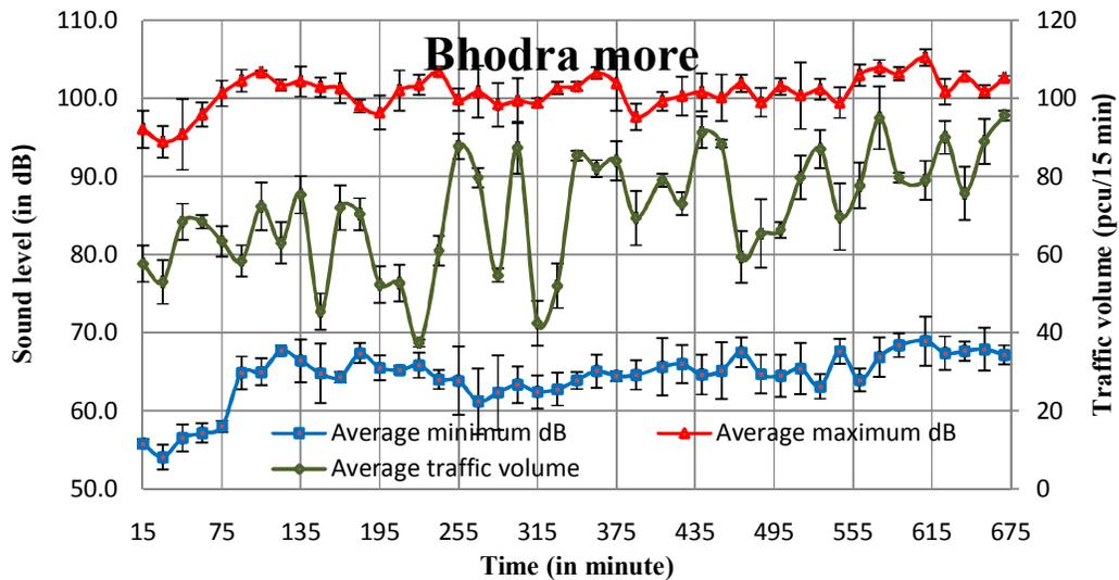
Figure 4: Sound level and average traffic volume with respect to time at Bhodra
