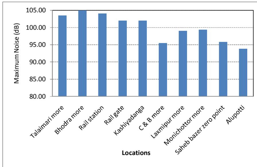
Figure 13: Average maximum noise level at different points
