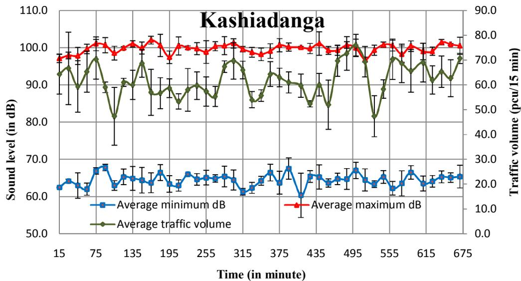
Figure 7: Sound level and average traffic volume with respect to time at Kashiadanga
