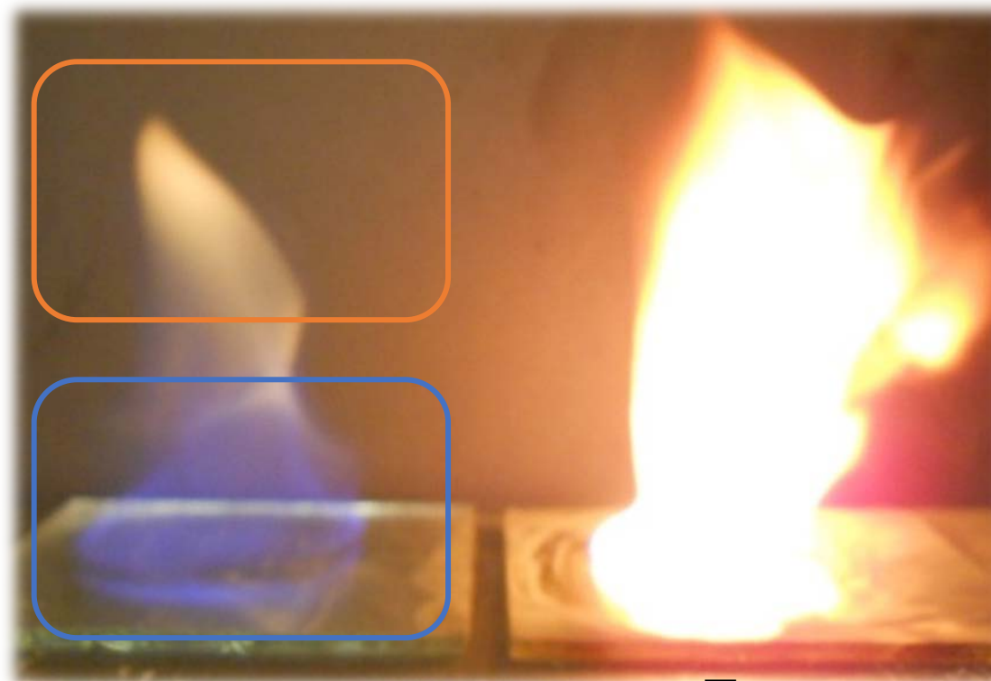
Pool fires of ethanol (left) and benzene (right) (photo: C. S. McEnally)
