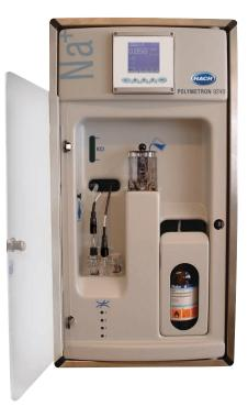
The POLYMETRON 9240 multi-channel provides low level sodium measurement in high purity water applications for up to four sample streams. With a detection limit of 0.01 ppb and a range of 0 to 10,000 ppb, this analyser is ideally suited for monitoring sodium in demineralised water, boiler feedwater, condensate and all parts of the steam/water cycle.
