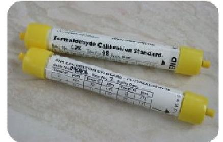
The calibration standard tube is used for checking and adjusting the calibration of the Formaldemeter. A known concentration of formaldehyde is generated in the headspace of the calibration standard, this is temperature dependent. Vapour can be sampled by the instrument to check accuracy and performance.
