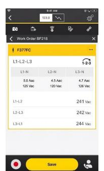
Fluke Connect pulls all data related to three-phase measurements including phase rotation and presents the full set of data for analysis at a glance.
