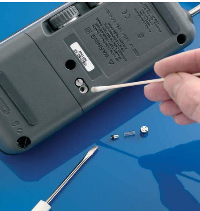
Cleaning the fluid trap in the Fluke-718 Calibrator is quick, easy and only requires a slotted screwdriver and cotton swab.
