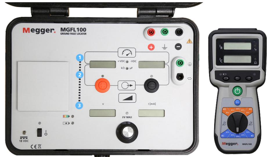
The MGFL100 is a battery ground fault locator. It can locate faults up to 400 kΩ. It can automatically identify real faults as well as leakage current. The unit will alarm when it locates the real fault.
