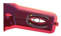
Megger clip being tested with IEC standard test finger for creepage and clearance.
