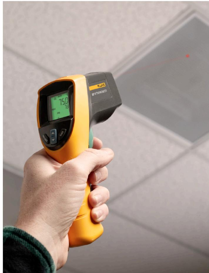
Measuring diffuser temperature.
