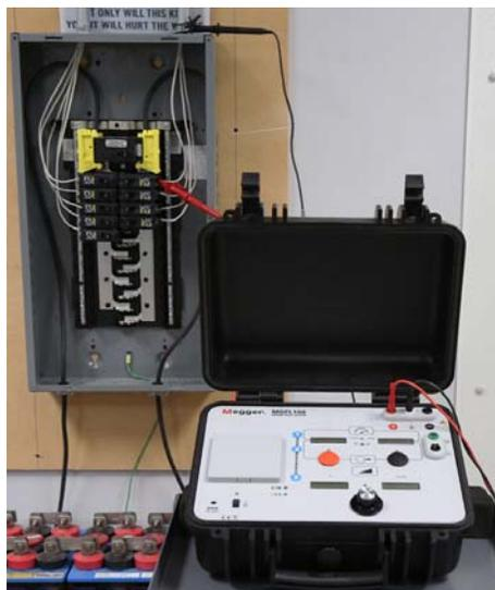
Turn on the MGFL100 output and apply a small current through each circuit. The transmitter will display the resistance and capacitance of each circuit.
