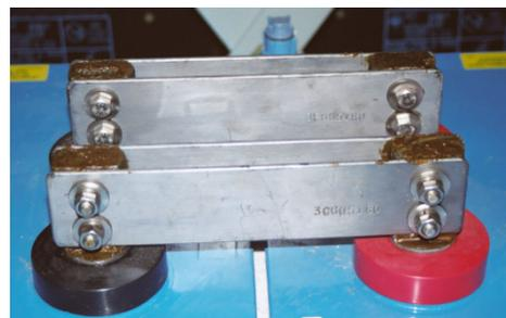
If you can take the measurement directly from the post of the battery, then both the terminal connection resistance and the inter-cell resistance is done at the same time. This is the recommended method per IEEE450.
