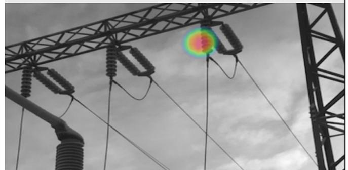
*System quickly provides PD type classification and PD pattern for further analysis*
