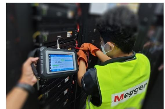
Figure 3: Testing of Individual Cell
