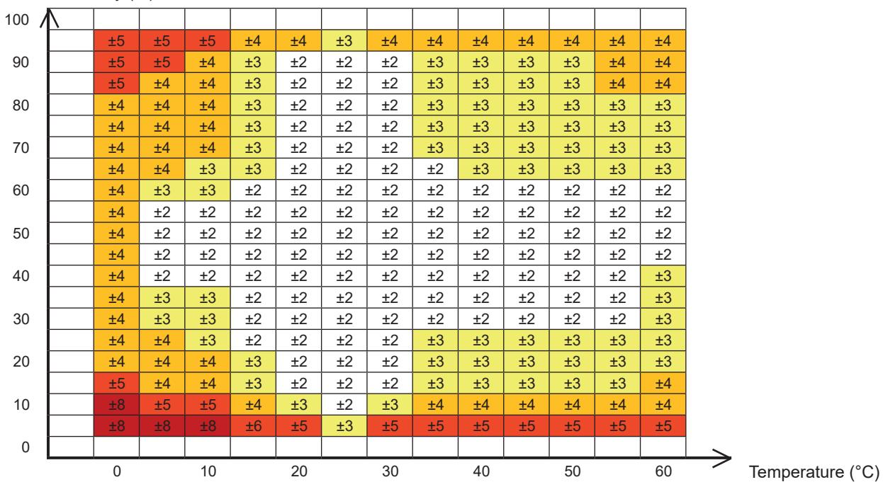
The relative humidity is highly dependent on the temperature. To calibrate the instrument, the two sensors (the reference sensor and the sensor of the instrument) must indicate the same temperature.
