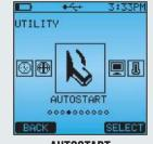
**AUTOSTART** Set the tester to activate a test process on contact.
