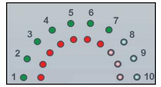
After the three seconds, the receiver starts to evaluate the signal level picked up by the identification clamp. It may take a few seconds until the receiver is able to clearly identify the incoming pulses and to indicate them appropriately.
