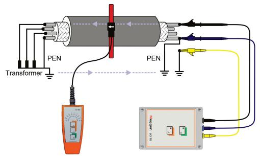
In order to minimize the risk of stray field induction, the flexible identification clamp (including the connection cable) must be connected at a distance of at least 10 cm from nearby cables. If there is not enough room for this, then at least the clamp closure and the connection cable should be positioned as far away as possible from the nearby cables (see diagram).
