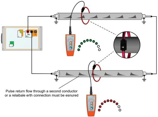
If no readable deflections are obtained, it should be checked (using a line locator) whether the cable to be identified is part of the bunch at all.
