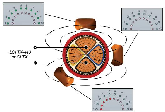
The following diagram illustrates the signal response when the sensor is moved along a four-core cable:
