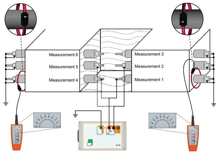
For this purpose, the identification generator is connected to one core and earth at the point where the cable is cut. Afterwards, the generator is switched on. For earthing, the screen of one of the other cables is used. When measuring at the near end of the cable, the core carrying the test current can then be easily identified by a deflection of the green LED bar (provided the clamp is aligned in the direction as shown in the figure).
