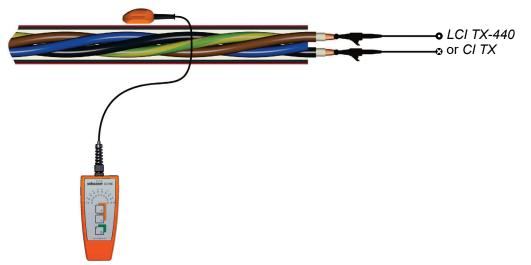
Process Due to the twist of the conductors along the cable, the fields formed around the two conductors are counter rotating. As the *TFS CI* sensor is moved along or around the cable to be identified, the green [1] and red [2] LEDs on the receiver light up in rotation.
