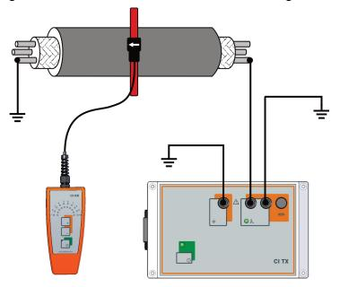
To identify live cables in combination with the *LCI TX* or *LCI TX-440* generator, the identification clamp should be placed around the cable with the direction arrow pointing towards the supply transformer as shown in the figure below:
