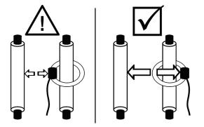
It is particularly important for the above instructions to be observed, if measurements are being taken from a multi-conductor cable and if the nearby disruptive object could be a phase of this cable that conducts return current. In the case of accessible individual phases (e.g. in low-voltage distributors), it is generally advisable to use the PAS CI sensor for phase identification (see section 6.3).
