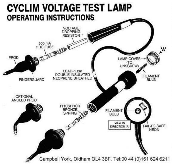
The Cyclim Voltage Test Lamp uses the brightness of a filament bulb to indicate the presence and variation of voltage. The neon in parallel with the filament bulb glows only when the bulb is broken or fitted incorrectly.
