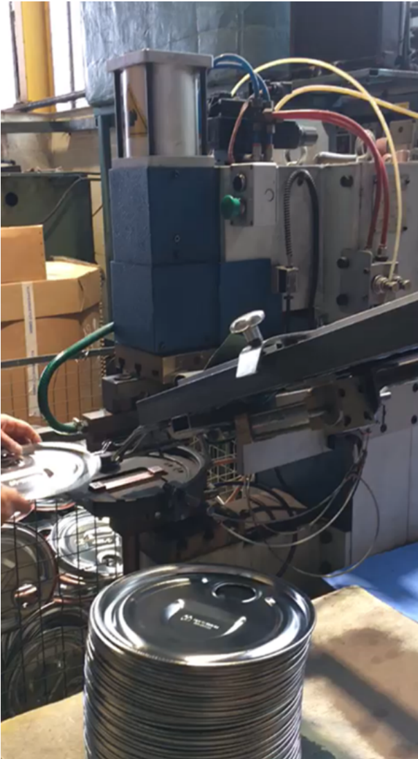
Figure 2: A spot welding machine used to weld handles on to metal lids
