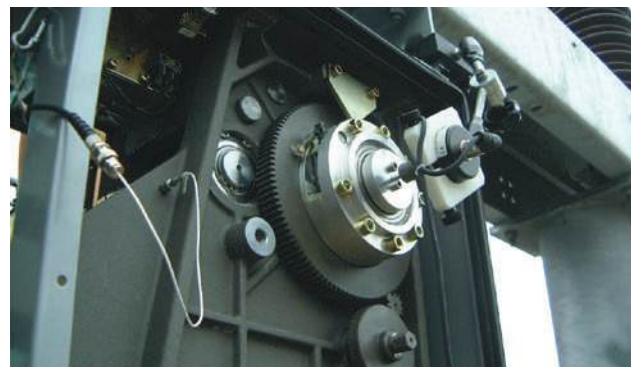
Circuit breaker operating mechanism with rotary motion transducer and accelerometer (for vibration measurement).
