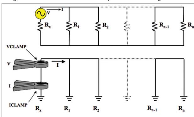
system testing applications. This method is also useful when there is insufficient space to perform a classic fall-of-potential measurement. In addition the units can be used to measure ground leakage or phase current.
