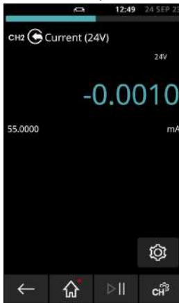
Figure 4-14: Measure Current on CH2 (Range \pm 55 mA)
