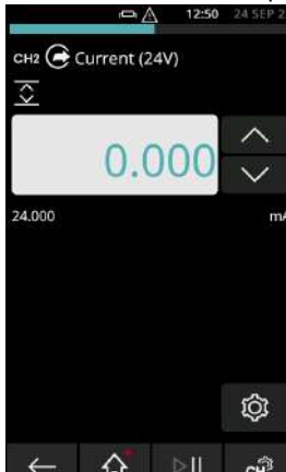
Figure 4-12: Source Current on CH2 with Internal Loop Power (Range: 0 to 24mA)
