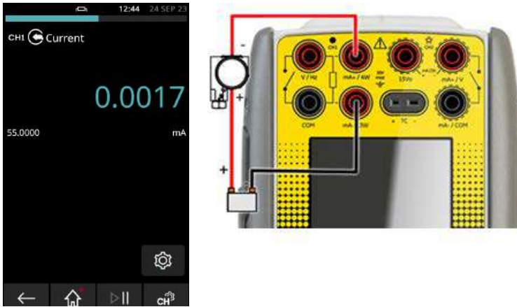
Figure 4-2: Measure Current on CH1 (Range \pm 55\text{mA} )
