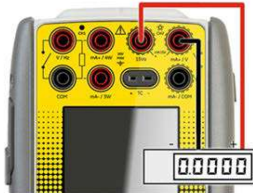
Figure 4-15: Connections for unregulated 15Vo Current Loop Output
