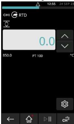
Figure 4-26: PT100 RTD Source CH1 4-Wire (Range -200 to 850°C)
