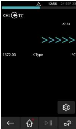
Figure 4-31: K-Type Thermocouple Measure CH1 (Range -270 to 1372°C)
