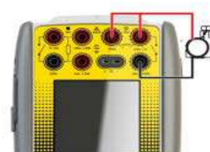
Figure 10-5: Example IS Connection Diagram FOUNDATION™ Fieldbus - Internal Network
