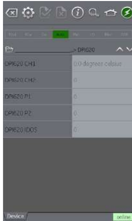
Figure 11-14: Profibus® Navigation Tree – DPI620G
