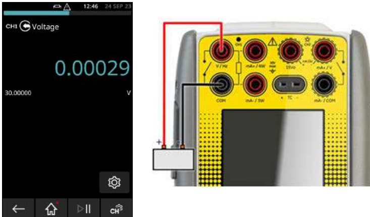
Figure 4-5: Measure DC Volts or DC mV on CH1, Range \pm 30V
