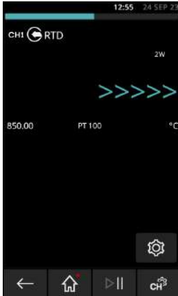
Figure 4-25: PT100 RTD Measure CH1 2-Wire (Range -200 to 850°C)
