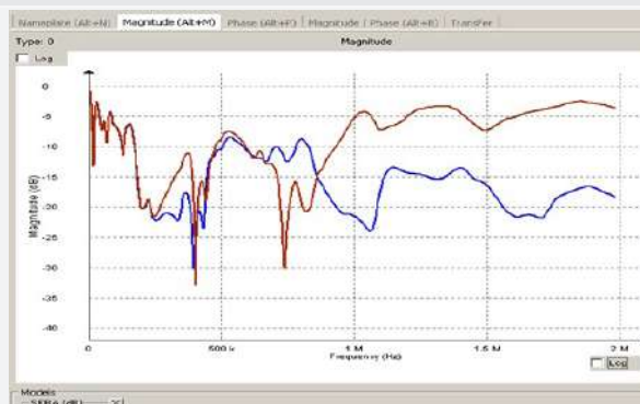
Bad connection can affect the curve at higher frequencies
