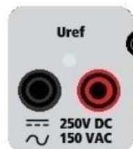
Figure 7 AC/DC AUX V4 Output Terminals
