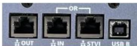
Figure 8 FREJA 546R Communication Ports
