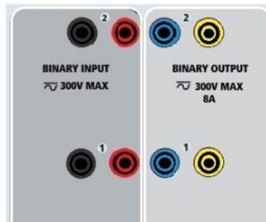
Figure 5 Binary Inputs and Outputs 1 and 2
