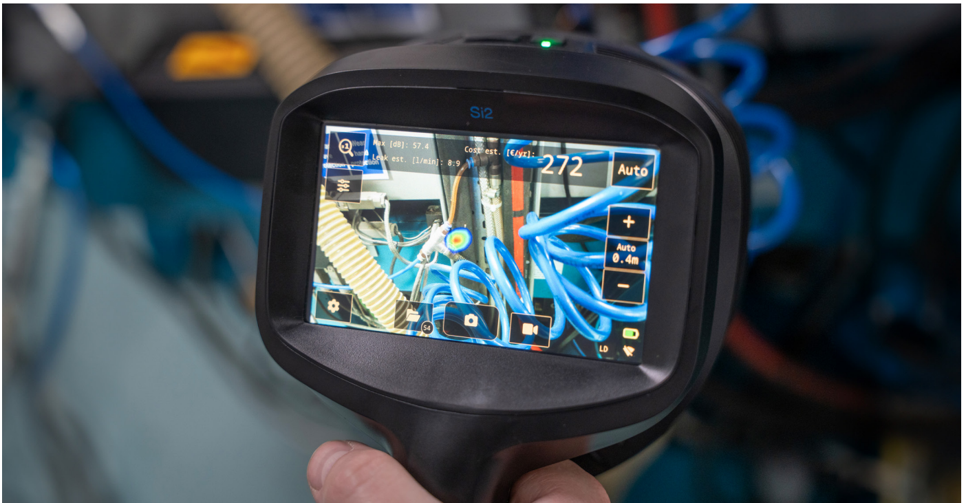
Acoustic imaging reveals hidden compressed air and industrial gas leaks, saving energy and improving uptime in glass production.
