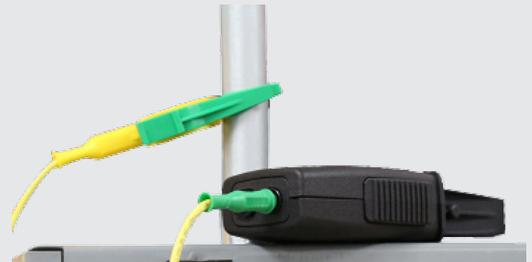
Place the current clamp on the positive lead of the transmitter after the IT Filter box.
