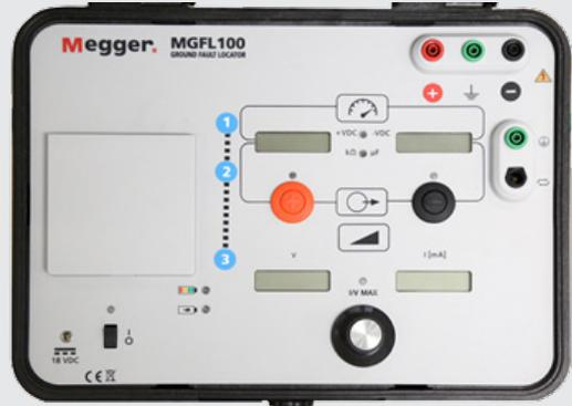
Connect the green terminal to the IT Filter box input.
