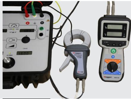
Connect the sync cable between the receiver and transmitter
