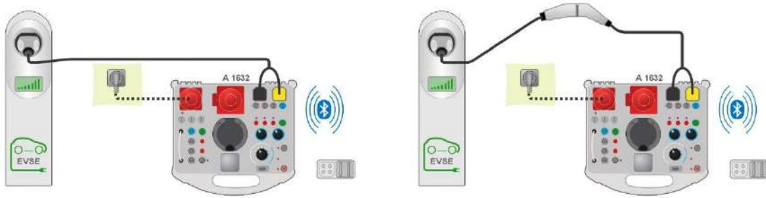
Diagnostic test - Connection to EVSE
