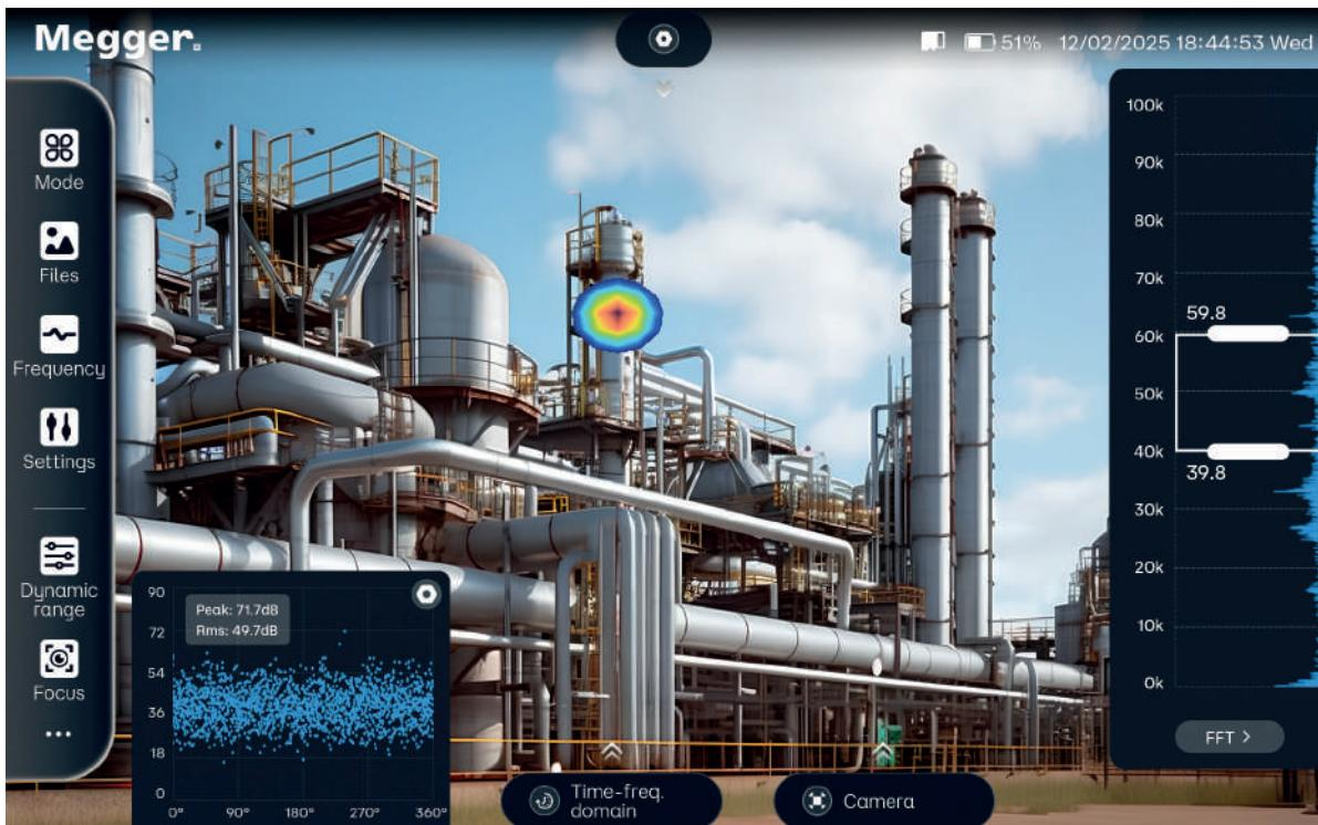
To edit the fundamental frequency of the electrical system being monitored, tap on **Settings** from the **Function Menu** and then on **Mode parameters** and then select **Partial discharge**. Users can select the frequency for the power grid according to its operating frequency, the default value being 50 Hz.
