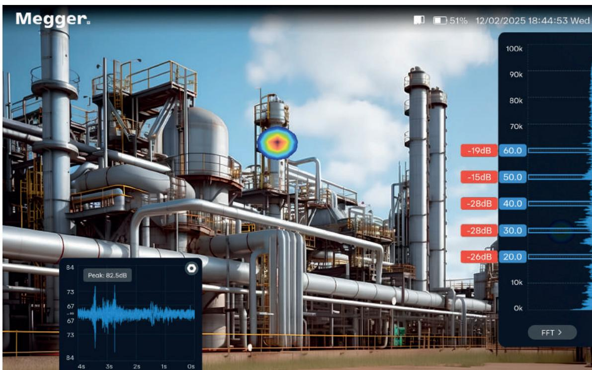
Tap on **Frequency** on the **Function Menu** to choose between single or multiple frequency measurement points. When multiple frequency points are selected, five frequency boxes will be displayed on the Frequency selection box on the right FFT display.
