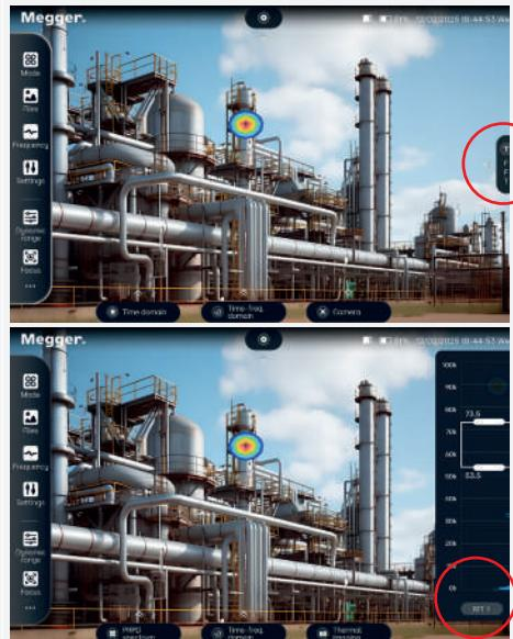
Tap the **○** on the top centre of the screen to view the **settings menu**. The menu can also be viewed by sliding the finger from the top of the screen downwards at any point.
